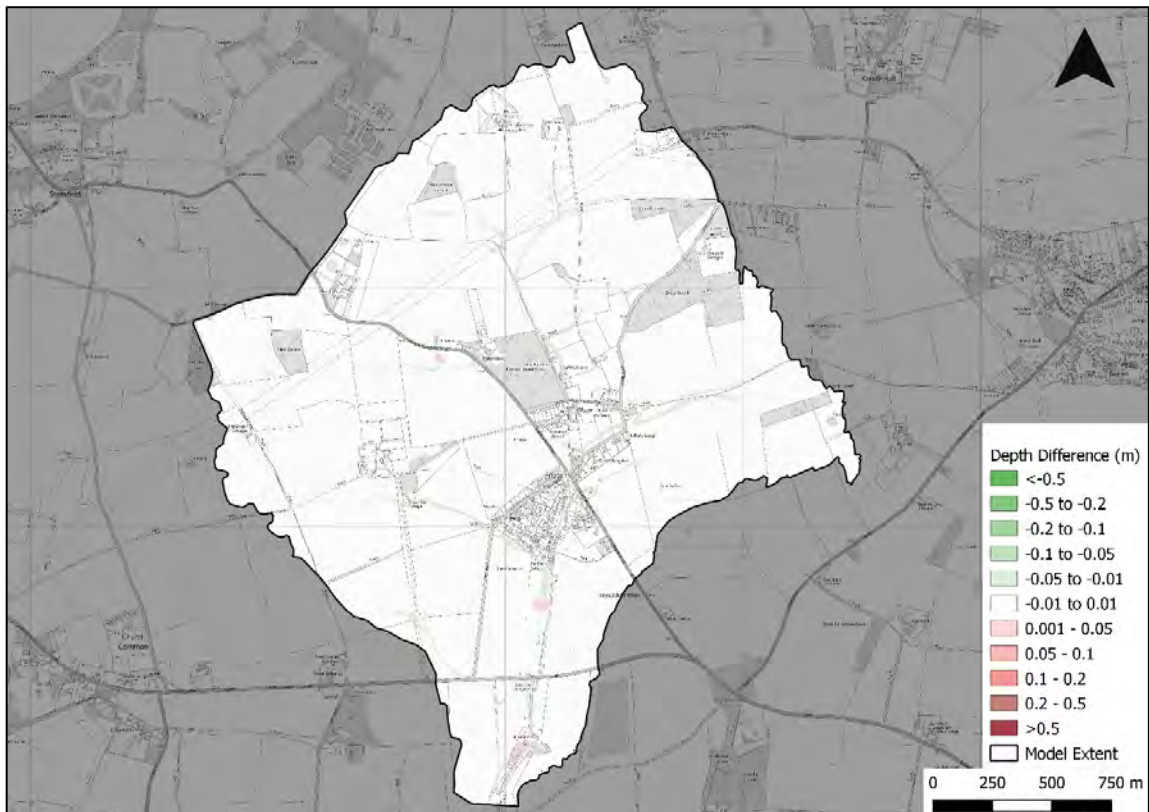
Figure 6-4 - Sensitivity: Floodplain Roughness -20% Vs Baseline, 1% AEP
